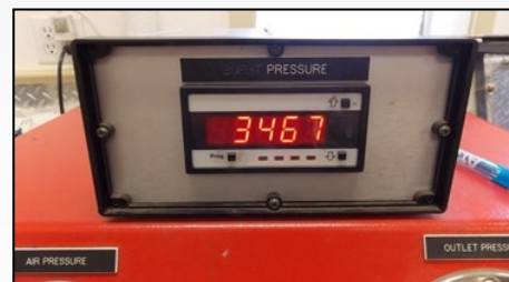
Hose failure at 3467 psi. (exceeding 4:1 safety factor)
